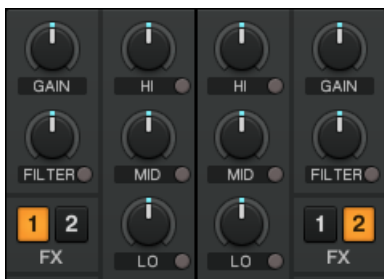
The FX Assign buttons on each channel
