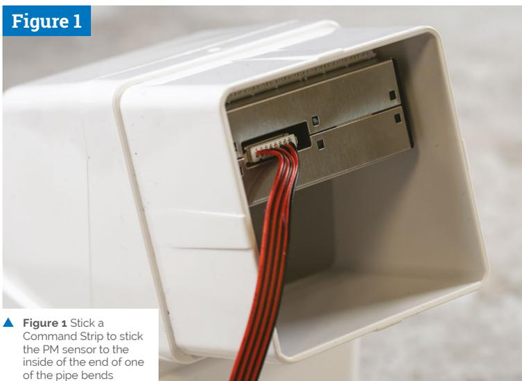
▲ **Figure 1** Stick a Command Strip to stick the PM sensor to the inside of the end of one of the pipe bends
