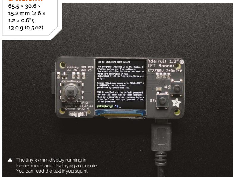
▲ The tiny 33 mm display running in kernel mode and displaying a console. You can read the text if you squint
