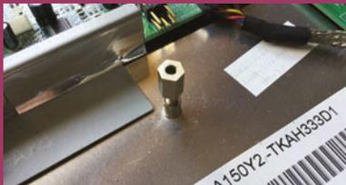
With the back off the VGA monitor, it revealed two short tapped pillars. We extended these with a 10mm M3 tapped pillar, fastened with a piece of M3 studding or thread cut from a longer bolt. This was the basic anchor for the system. It was fastened to a length of 30x12 aluminium channel of 3mm thickness that spanned the whole width of the frame. The channel walls were trimmed to fit flat.
