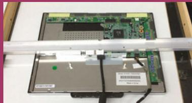
At each end, a piece of 20mm angled aluminium was mounted so that it could be bolted onto the frame with two M3 bolts. Holes in the top were used to fasten this to the long channel to make a secure fit. We found it a bit fiddly to hold the nuts on the underside of these right-angled brackets, so we fastened them on the underside with hot-melt glue to allow easy assembly and disassembly.
