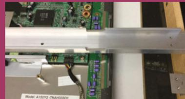
Slots were cut in the wall of the channel to allow cables to pass through, and also allow clearance for some components on a side board. Don't cut too deep or you'll start weakening the beam somewhat – in the long run, that would be bad for the overall structural strength of the mirror, and that wouldn't make your life easier in the way we want.
