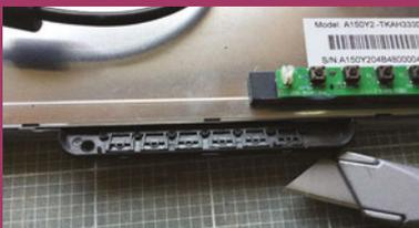
The monitor's control buttons were removed from the front panel and hot-melt-glued on a piece of foam mounted to the back of the monitor. Then the control panel mount was removed by careful use of a knife; the monitor's shape was a clean rectangle and the mounting foam for the surrounding was a lot easier to cut. The surrounding mount was cut from black A3 foam in two pieces.
