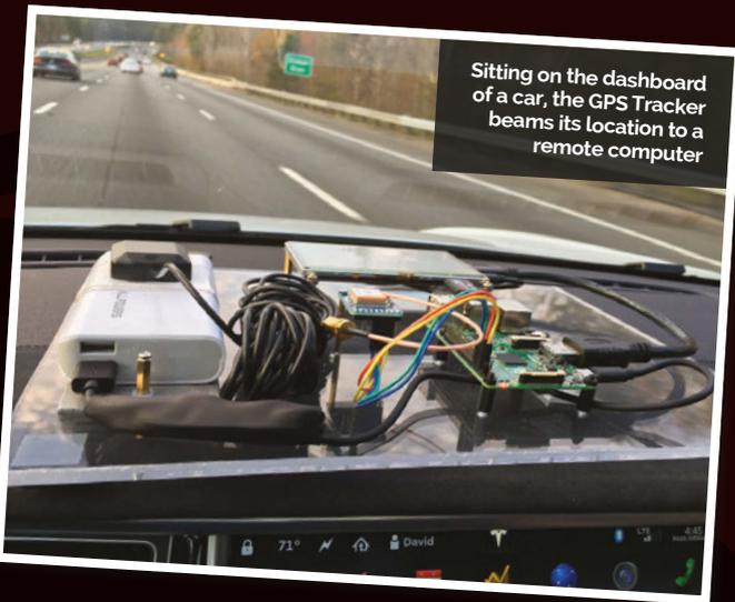
battery holder. Wires are soldered to the board and then connected to the GPIO pins on the Raspberry Pi. "If you've never done any soldering before, I recommend you get some spare header pins, a breadboard, and a perma-proto board to practise on," says David. A uFL-to-SMA connector is then used to connect the Ultimate GPS Breakout board to an antenna.
