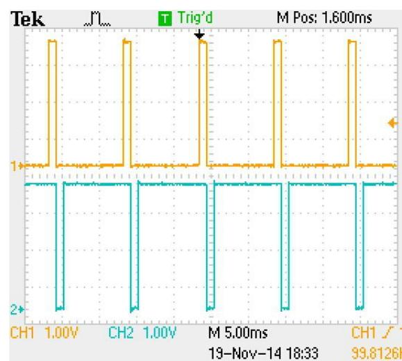
**Figure 1** - Pulse width modulation signals
