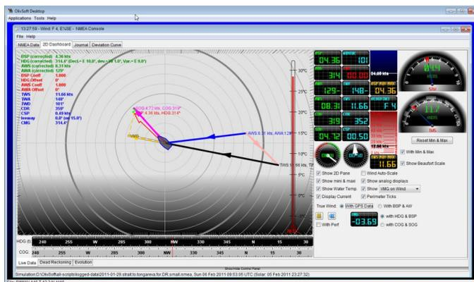
I have recently enhanced it to run in headless mode (i.e. without a graphical user interface), to run on the Raspberry Pi. When headless, the role of the Navigation Console is to read and compute the data, optionally save to a log, and then re-broadcast them on one or more channels. For such a re-broadcasting to happen, the Raspberry Pi creates its own ad-hoc wireless network. Other devices will join this network, and will then have access to the re-broadcasted data.
