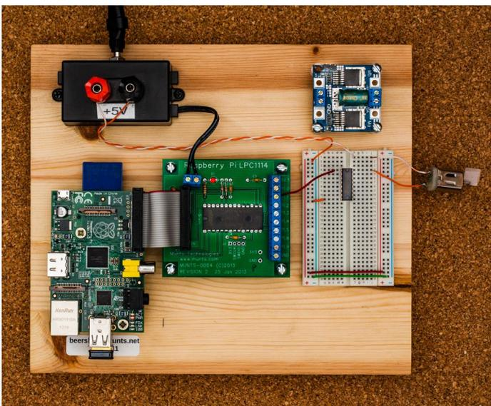
Figure 3 - Small DC motor test stand
