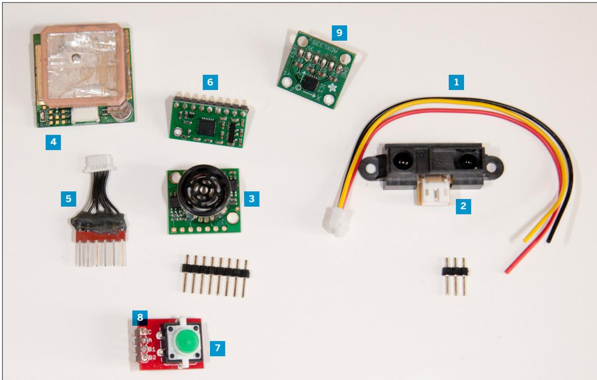
**Figure 8-1.** New parts for this chapter: **1.** Sharp GP2Y0A21 IR ranger **2.** JST pigtail for IR ranger **3.** Maxbotix LV-EZ1 ultrasonic ranger **4.** EM-406A GPS receiver **5.** Interface cable for EM-406A **6.** LMS303DLH digital compass **7.** LED tactile button **8.** Breakout board for button **9.** ADXL335 accelerometer. Don't forget plenty of male header pins for the breakout boards.
