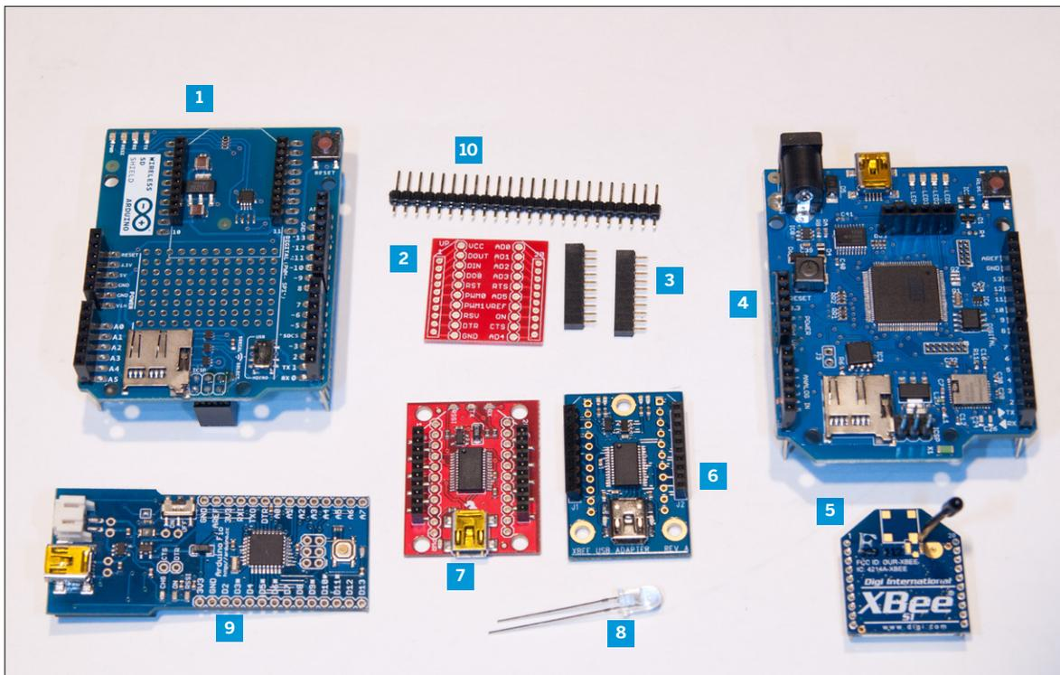
**Figure 6-1.** New parts for this chapter: **1.** Arduino wireless shield **2.** Spark Fun XBee breakout board **3.** 2mm female header pins **4.** Arduino WiFi shield **5.** Digi XBee 802.15.4 OEM module **6.** Adafruit XBee-to-USB adapter **7.** Spark Fun XBee Explorer **8.** Infrared LED **9.** Arduino Fio. Don't forget plenty of male header pins for the breakout boards.
