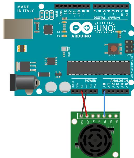
▶ This sketch is similar to the infrared ranging sketch in Project 15. It reads the sensor and converts the results to a voltage, then converts that to a distance measured in centimeters. The conversion formula again gives only an approximation.
