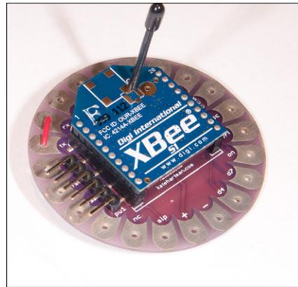
back into the receive pin, where they will be sent out again as transmissions. Figure 7-14 shows the circuit. You could also use a LilyPad XBee, XBee Explorer Regulated, or any USB-to-XBee serial adapter. Just tie the transmit and receive pins together, and attach a battery to the voltage input of the regulator.
