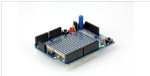
The ultimate open source prototyping shield for Arduino & compatible microcontrollers. Create your circuits the way you want, and easily changes without having to solder.
