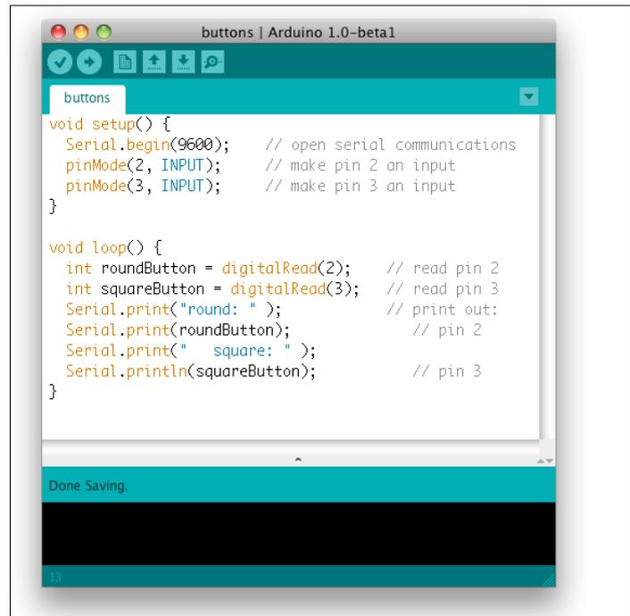
an Upload button as well. Verify compiles your program to check for any errors, and Upload both compiles and uploads your code to the microcontroller module. There's an additional button, Serial Monitor, that you can use to receive serial data from the module while you're debugging.
