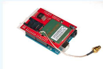
Two ways to get GPRS to a microcontroller: the Telit GM862 evaluation board breaks out all the pins of the module to 0.1" spacing; the SM5100B shield breaks out the serial pins of its module to the Arduino's serial pins.
