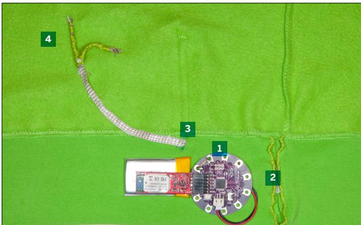
**Figure 10-21.** The layout of the hoodie components on the inner lining: 1. The LilyPad Arduino and the battery are actually inside the bottom band of the garment, inserted through 2. the large cut on the right. The conductive ribbon comes out of the bottom band through 3. the small cut, and goes to 4. the pocket contacts at the top (opposite side of the garment).
