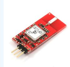
GPS MiniMod with GR10/MN1010 receiver. Smallest I could find. Takes a long time to acquire a signal.
