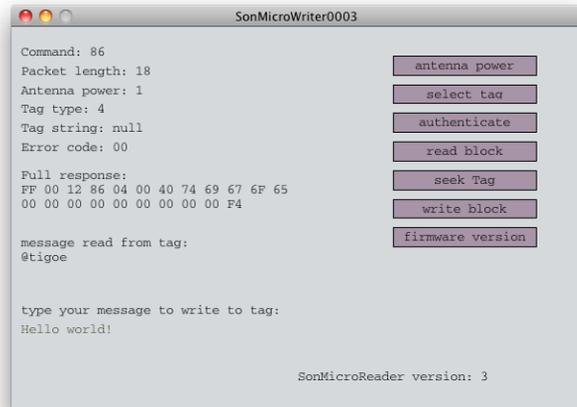
**Write to It** This Processing sketch lets you read from and write to the memory on a Mifare tag using the SM130 RFID reader. It uses the SonMicroReader library for Processing.
