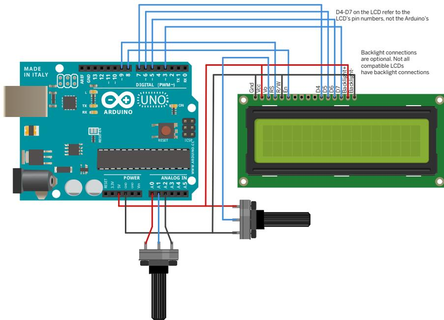
D4-D7 on the LCD refer to the LCD's pin numbers, not the Arduino's
