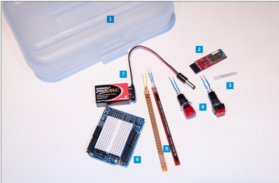
**Figure 2-1.** New parts for this chapter: **1.** Project box **2.** Bluetooth Mate **3.** RGB LED **4.** Pushbuttons **5.** Flex sensors **6.** Prototyping shield, **7.** 9V battery snap connector and female power plug. Don't forget plenty of male header pins for the breakout boards.
