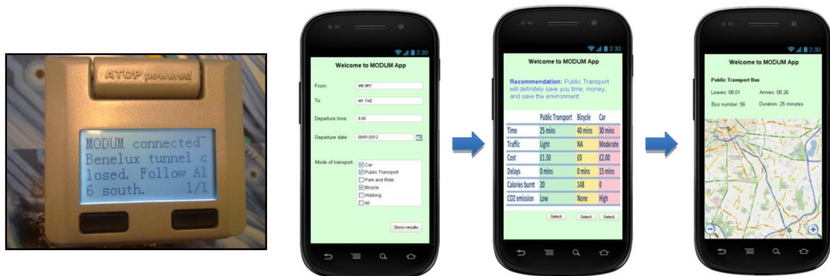
Fig. 7. Left: the ATOP device installed in a vehicle, showing how text messages can be sent to a user in real-time. Right: the graphical user interface of the MODUM end-user prototype running on an Android smartphone.
