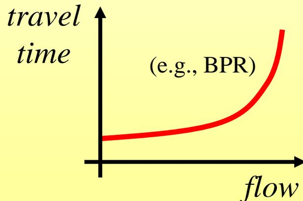
It is difficult (*but necessary*) to capture the concept of “**capacity of a road**” !
