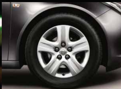
❸ Stalen designvelg, 7 J x 17, 5 spaken, bandenmaat 225/55 R 17 (QR8).
