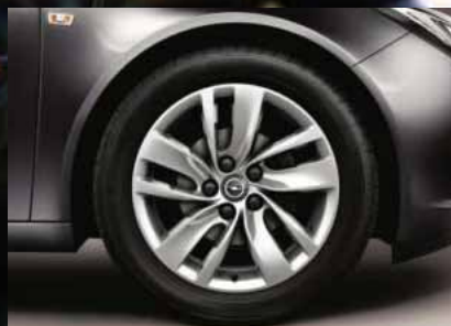
❺ Lichtmetalen velg, 8 J x 18, 5 spaken, Sport Design, bandenmaat 245/45 R 18 (PXR).
