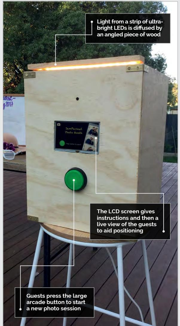
Light from a strip of ultra-bright LEDs is diffused by an angled piece of wood
