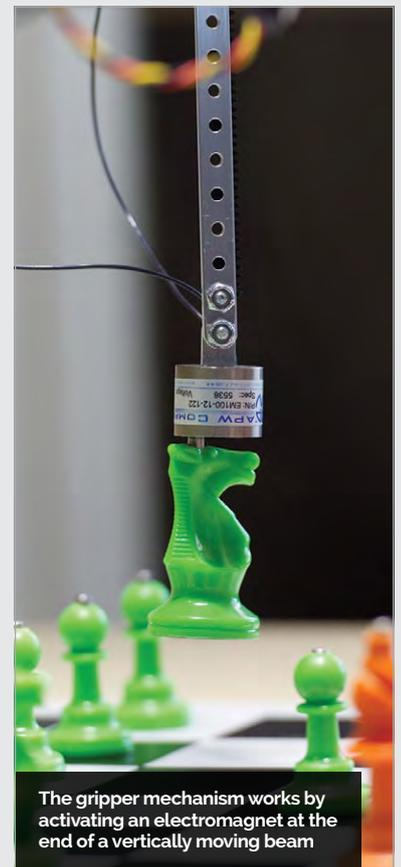
The gripper mechanism works by activating an electromagnet at the end of a vertically moving beam
