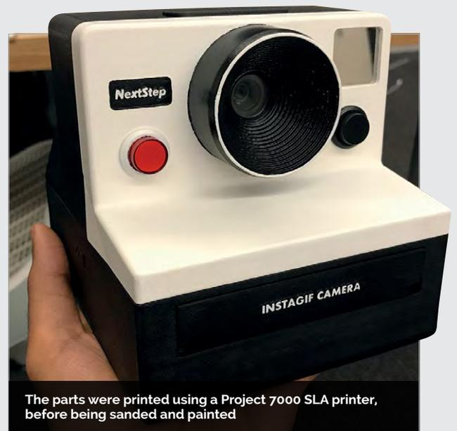
The parts were printed using a Project 7000 SLA printer, before being sanded and painted
