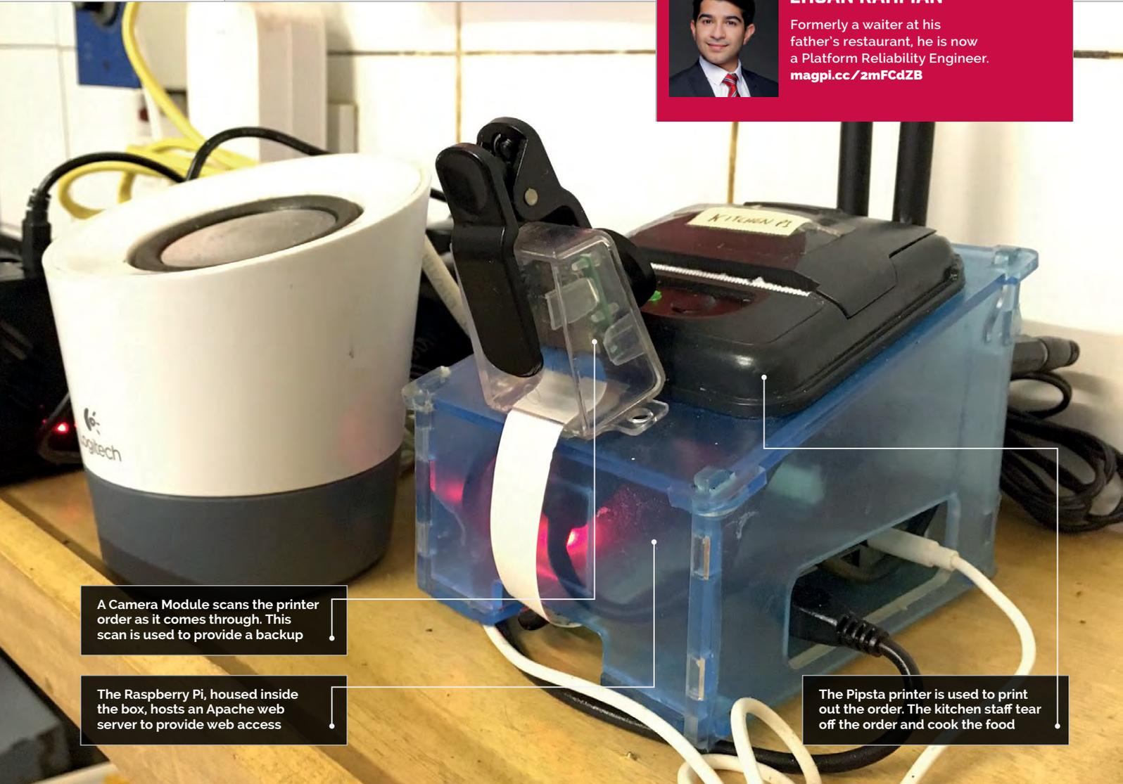
A Camera Module scans the printer order as it comes through. This scan is used to provide a backup
