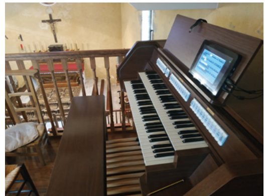
▲ Digital organs have been used in place of pipe organs within churches for a while, but damp and the scarcity of spare parts mean they're not lasting as long
