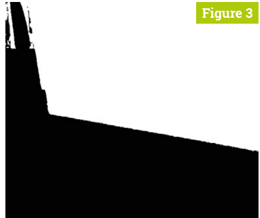
▲ Figure 3 Example of a masked or thresholded image. Pixels are only on (white) or off (black)
