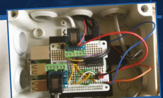
Above The Raspberry Pi is fitted in a large box with holes on the side to enable access to the external components. A 3D-printed mount is used to keep the Raspberry Pi from moving around
