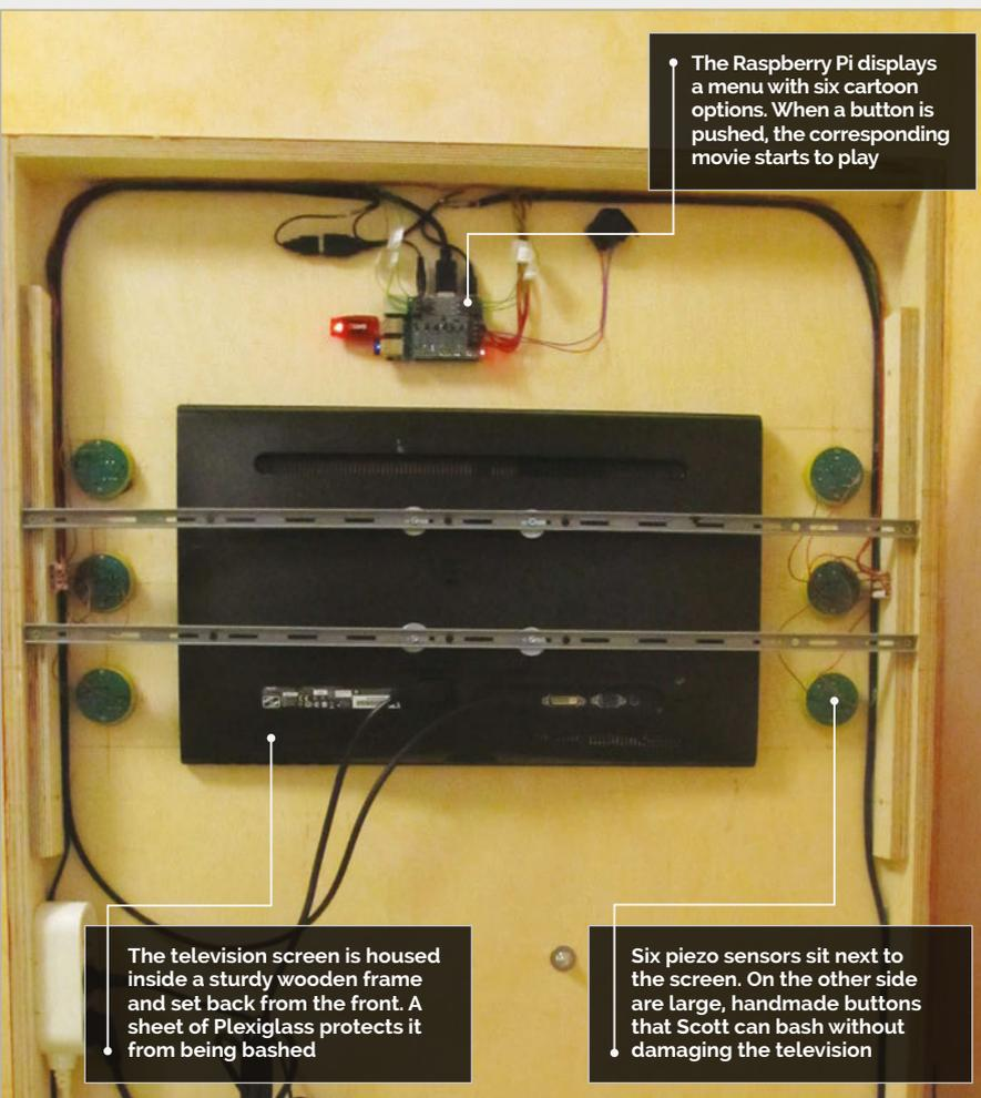
Plexiglass in front of the display is the solution. “It wasn’t complicated to build,” says Alain. “With a jigsaw, a drill machine, and a little table saw, all is possible.
