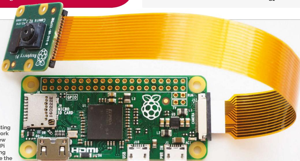
All the existing cameras work with the new Raspberry Pi Zero, as long as you have the adapter cable
