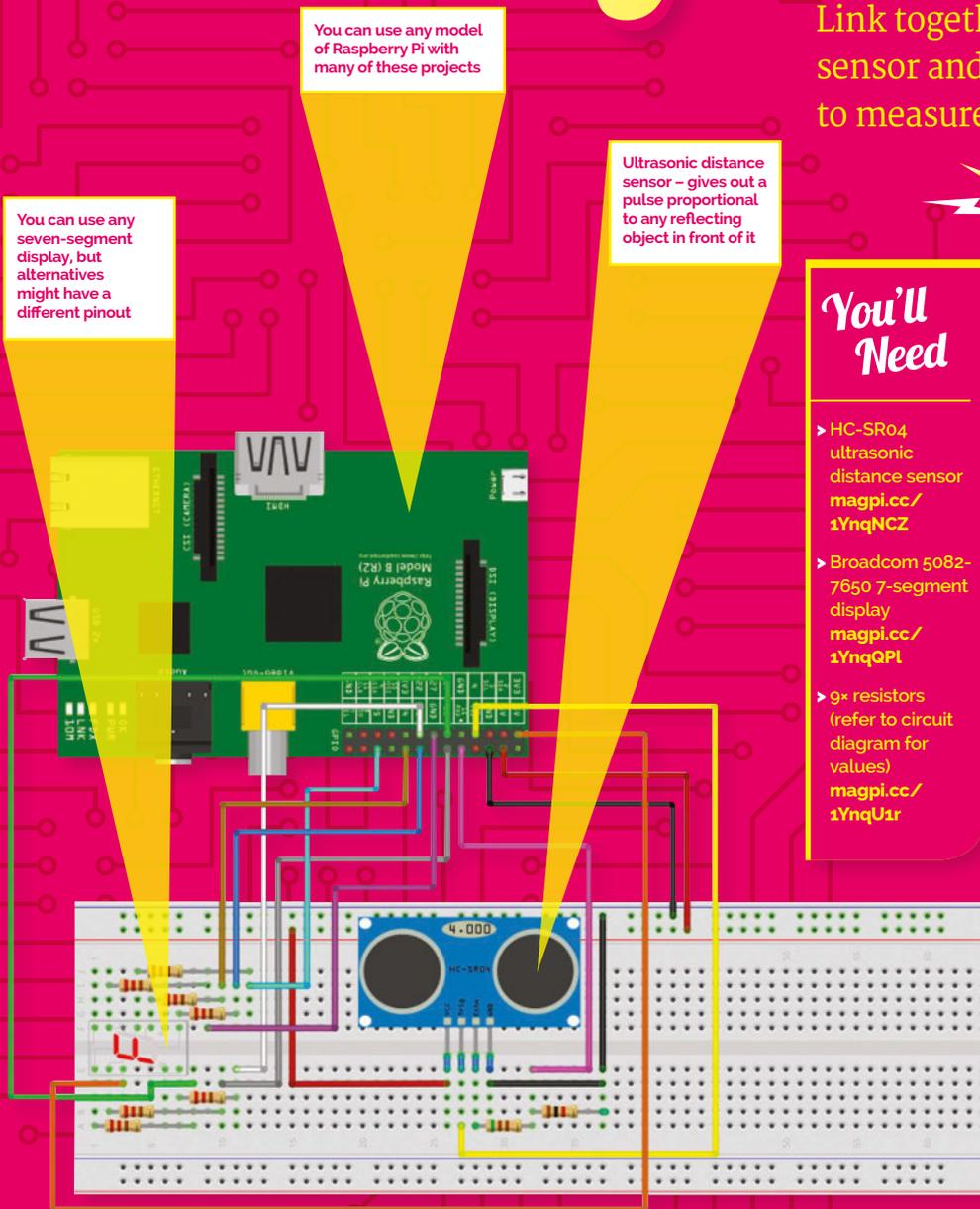
You can use any seven-segment display, but alternatives might have a different pinout
