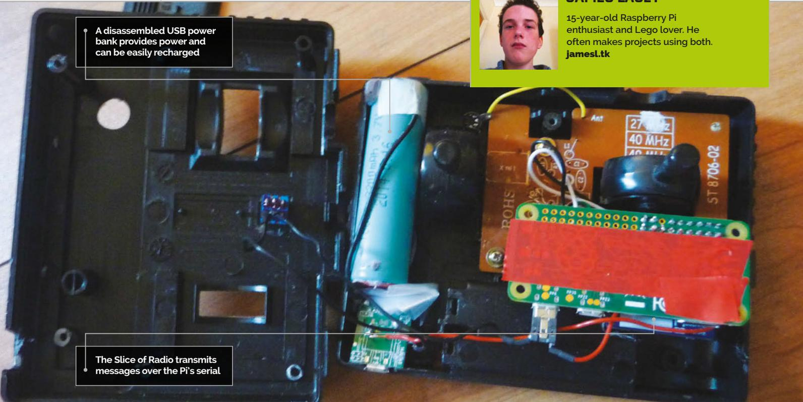
A disassembled USB power bank provides power and can be easily recharged
