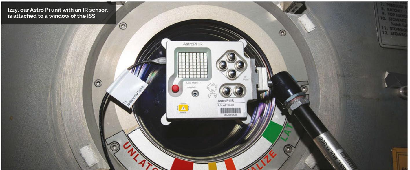
Izzy, our Astro Pi unit with an IR sensor, is attached to a window of the ISS
