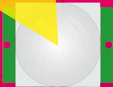
**N**eed to protect your room or precious items from ne'er-do-wells or nosy family members? With just a PIR motion sensor and a buzzer wired up to your Raspberry Pi, it's very simple to create an intruder alert. Whenever movement is detected in the area, a loud beeping noise will raise the alarm. To take things further, you could add a flashing LED, an external speaker to play a message, or even a hidden Camera Module to record footage of intruders.
