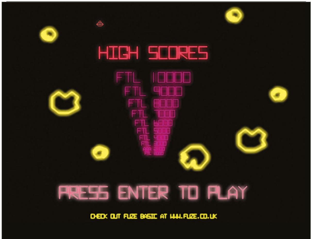
distance between each asteroid and the player ship. If it's less than the radius of the ship and the rock, i.e. touching, then it's a crash! When we hit a big rock, we want it to break into two, then again for a medium one; if it's a small one, there's just the explosion, so we use `DEF PROC silvoidSmash` to do this.
