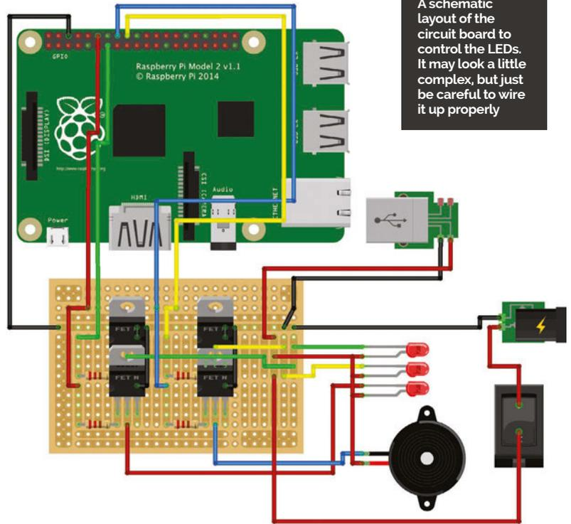
A schematic layout of the circuit board to control the LEDs. It may look a little complex, but just be careful to wire it up properly
