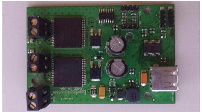
As mentioned previously, the SmartDrive allows the Raspberry Pi to control up to two high current motors. The SmartDrive is controlled by the Raspberry Pi using the I<sup>2</sup>C interface.
