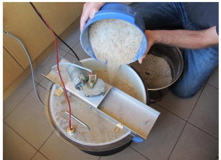
The first step in brewing is the mashing. During this step the starch of the malt is converted to sugar and extracted from the malt so the wort is obtained. (Wort is the liquid extracted from the mashing process during the brewing of beer.)
