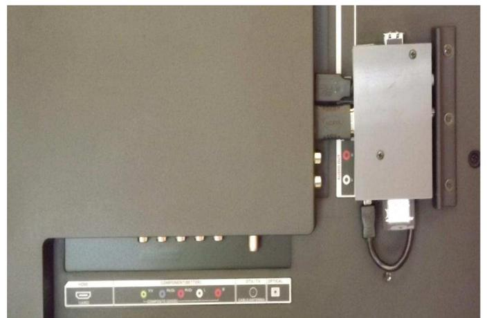
While any HDTV can be used, the example HDTV is particularly good as it has a USB connector sufficient for powering the Raspberry Pi. It also has a recessed area on the back for attaching the Raspberry Pi, which allows for flush wall mounting. Finally it has a narrow, clean bezel which makes a nice frame.
