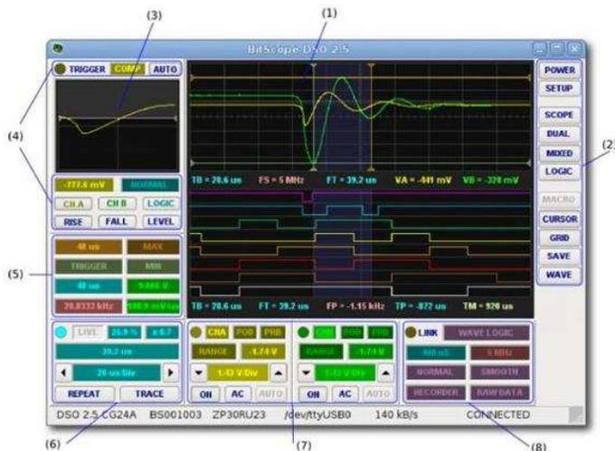
**Fig. 1:** BitScope DSO software main screen elements
