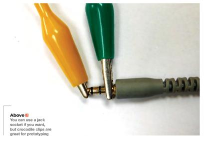
Before we dive into the code, let's take a look at the hardware. If you're using a board without dedicated audio hardware (such as a Pico), you just need to connect a pair of headphones between one of the GPIO pins and ground. The easiest way to do this is to clip crocodile clips onto the headphone jack.
