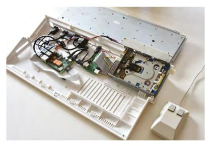
No soldering was needed for this build. The components are simply connected up
