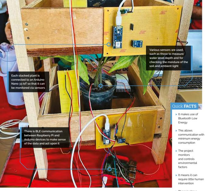
the IoT platform ThingSpeak. "ThingSpeak is useful for visualising data from sensors in realtime which provides valuable insights to farmers," he continues. "A user-friendly interface makes it accessible to those without extensive technical knowledge and providing a fault tolerance to the system."
