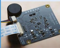
CinePl XL uses a OneInchEye sensor. Code for it is built on top of Raspberry Pi OS 64-bit Lite using libcamera-apps / libcamera. Setup instructions for the original CinePI are at github.com/CinePl.
