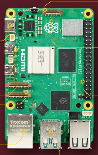
This small connector is a Raspberry Pi connector for PCle Expect to see exciting peripherals very soon
