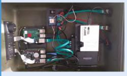
A UV spectrometer, WittyPi HAT, and network drive manage data and send it back to the volcano monitoring team for analysis.
