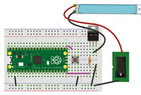
Figure 2: A breadboard prototype with a COB LED light strip and a connector for a 5V power supply
