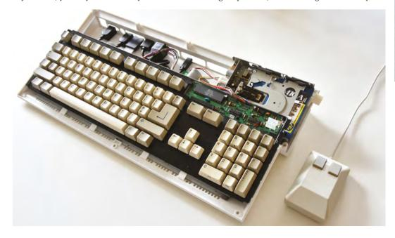
The Amiga 500 keyboard fits neatly on top of the components with plenty of space available in the case
