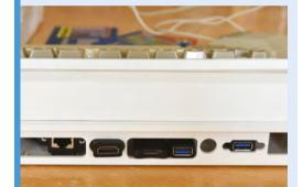
With an assortment of cables, Rob was able to add various ports to the back of the 'Amiga' by ensuring the ends were accessible via the holes. They include HDMI, USB-C, and USB-A, meaning peripherals can be connected to the machine.
