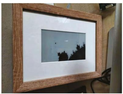
The maker kept the assembly pretty simple, cutting a small hole in the picture frame's back mount panel to slip the display HAT's ribbon cable through, with the project's Raspberry Pi left free-floating behind it. The e-ink display itself fits snugly inside the frame, with a card mount providing a little breathing space between the display and the glass.
