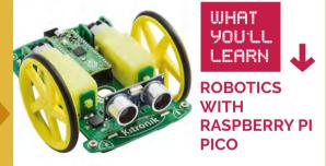
Similar to the EduKit #3, this is the Pico equivalent that allows you to quickly and easily build your own rover that can be programmed to work autonomously. It even comes with a chassis. Pico is great for robotics even if it it's not as powerful as a full-sized Raspberry Pi.
