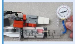
A motorised LEGO gearing system adjusts the ballast syringe. A hose sucks in water and draws water into the syringe chamber. Buoyancy remains constant while the extra weight of water increases the gravitational pressure.
