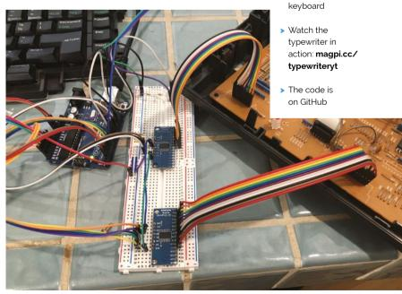
A voltage divider circuit has been created so that the 5V output of the Arduino is at a safe 3.3V level for Raspberry Pi
