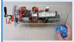
A radio board and controller culled from a cheap toy provide a user-friendly remote control, powered by Raspberry Pi, with no need for a dedicated battery.
