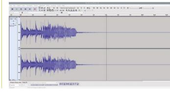
This twelve-second jingle only has between six and seven seconds of audible sound. Using Audacity, you can trim it.
