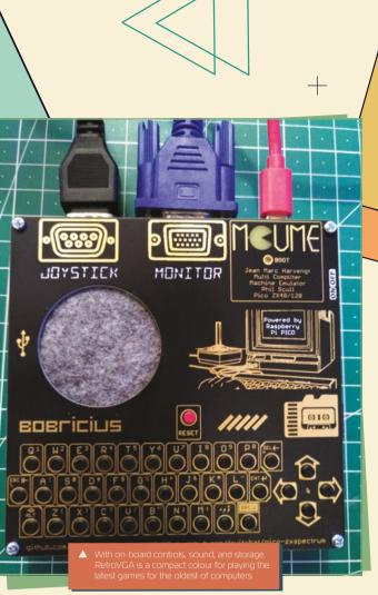
It uses different GPIO to VGA connections, which are documented in the project repository at magpi.cc/picovga.
