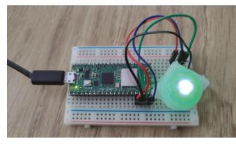
The cover from a PIR sensor makes a decent diffuser for the light from the RGB LED
