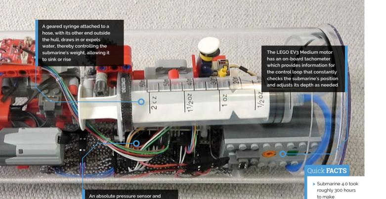
laser sensor monitor the submarine's depth, while a Raspberry Pi Zero 2 W
