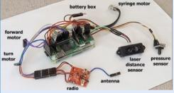
As well as a food syringe and LEGO gear wheels, you'll need a Raspberry Pi Zero 2 W with 16GB microSD card, a LEGO EV3 Medium motor with tachometer, and a 27MHz radio controller.
