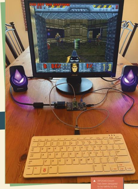
functionally identical to the "VGA, SD card, and audio demo board" described in Raspberry Pi's 'Hardware Design with RP2040' documentation (magpi.cc/rp2040hardware). Sanderson notes, "It is a lot easier to use the VGA Demo Base, though!"
