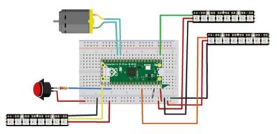
Figure 1 The components are arranged in sections to make separation easier. Bottom left is the handle, bottom right is the tank, top right is the wheels, and then the motor is on its own
