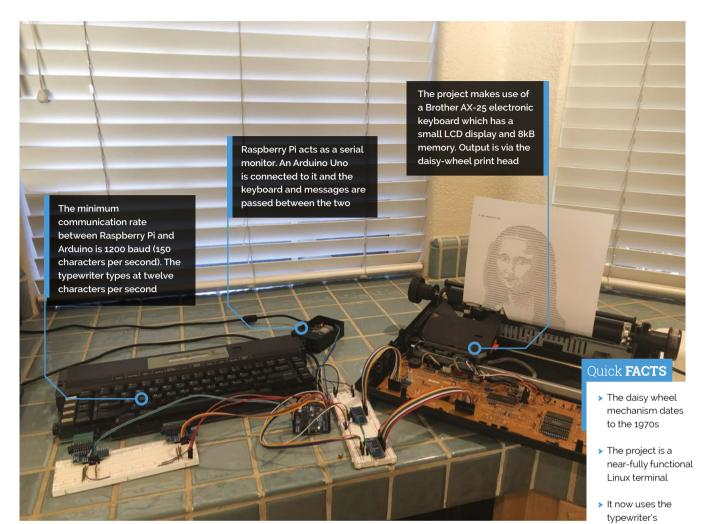
After that was working, he connected the typewriter's own keyboard to the Arduino. "The Arduino checks each pair of pins one at a time using the multiplexers until it detects that a key has been pressed," Riley says. "Once it does, it sends that key to the Raspberry Pi computer for processing."
