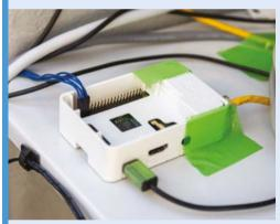
A humidity monitor was set up for the telescope because the DAQ [data acquisition] system originally had no roof. A Raspberry Pi initiates the dome closure whenever humidity gets too high.
