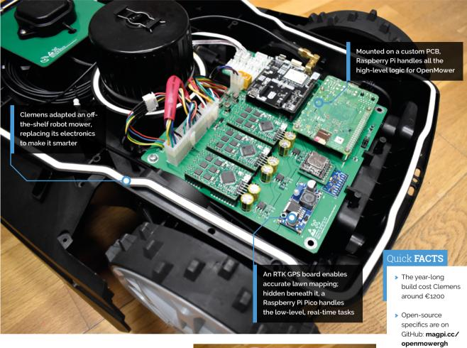
Clemens also added precise RTK (real-time kinematic positioning) GPS to his bot which, he says, makes it very flexible, efficient, and allows for better control. It even means that you can have multiple areas mowed separately. "You can plan an efficient path which covers the area, and even pause and resume exactly where you left off."
