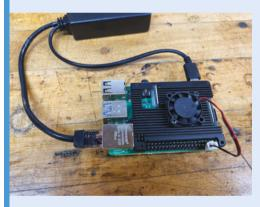
The Power over Ethernet card and PoE adapter, plus a power supply with fan, ensure BirdNET-Pi can be used to remotely record and identify bird species.
