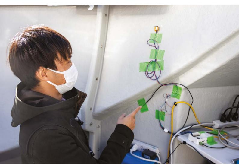
Shunsuke Honda points out the pera-pi Raspberry i sensor checking on the humidity and temperature within the telescope dome
