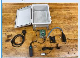
A waterproof housing, Raspberry Pi, microphone, fan, and cables make up the basics of an in-the-field BirdNET-Pi station. Photos from Bill Powers' setup (magpi.cc/birdnetbuild).
