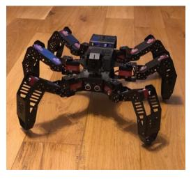
it a Meccano-like appearance. This also gives you some idea of how robust and well-constructed this clever hexapod is. The robot's HD camera head can rotate through 140 degrees while observing its immediate surroundings, picking out faces and signalling recognition by waving a leg.
