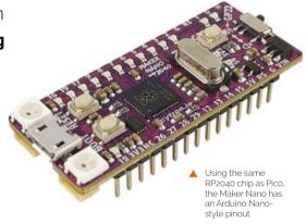
cool colour-changing effects can be achieved. In addition, 14 of the digital pins have tiny blue status LEDs that may well prove useful when troubleshooting I/O connections for circuits.
