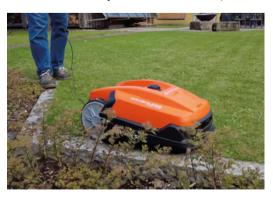
By first driving the robot around the lawn perimeter, and obstacles such as trees, a GPS map is built up for automatic mowing
