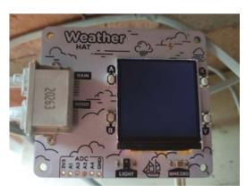
Mounted on a Raspberry Pi Zero (hidden beneath), the Weather HAT has on-board BMF280 and light sensors
