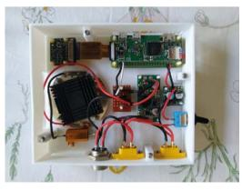
A lot of components are stuffed into the box. Emilio enjoyed figuring out the circuitry to control the IR LEDs
