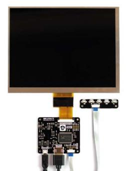
The Pimoroni 8-inch HDMI IPS LCD Screen Kit includes a display driver board, which sits between the computer and the screen
