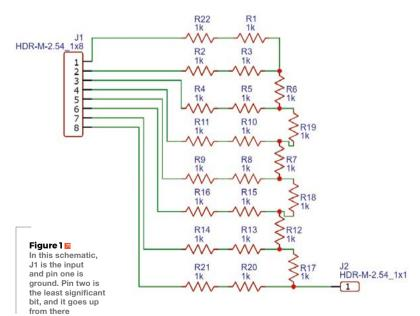
For example, if we wanted to output the lowest possible voltage (other than 0), we'd just switch the first digital output on. If we wanted to output the highest possible voltage, we'd switch them all on. This gives us 127 possible voltages we can output (representing every combination of digital outputs turned on).
