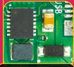
**7 POWER MANAGEMENT** These chips form the power management for Raspberry Pi Pico, which is fixed at 3.3 V.
