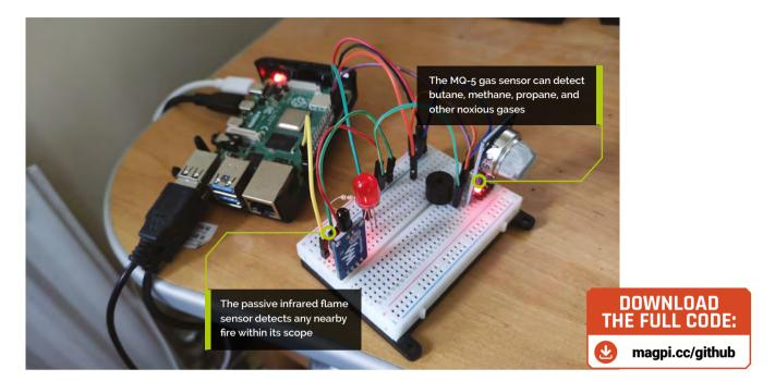
our code, we import the Button method from it. We'll use this to sense when the digital output from the sensor is high, in effect the equivalent of a push-button being pressed. As it's connected to GPIO 21, we assign the flame object to this with flame = Button(21)
