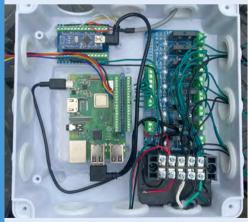
For more detailed monitoring, add a relay board for AC control, GPIO buttons for a physical interface, environmental sensors, and LED status displays, as per Oasis-grow's full configuration.
