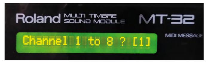
Above The MT-32 defaults to receiving MIDI on channels 2-9; press the MASTER VOLUME and 5 buttons at the same time, then tap 1 to switch it to a more conventional channel 1-8 configuration
