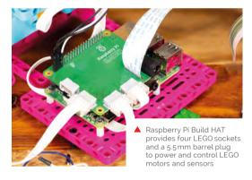
is included in the latest LEGO Education SPIKE Prime portfolio (version 45681; £362 / \$340; magpi.cc/spikeprime). With the Build HAT attached, Raspberry Pi can control up to four LEGO motors and/or sensors using Python code.
