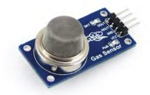
▲ The MQ-5 gas sensor can detect several noxious gases in the air and is highly sensitive
