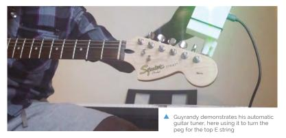
pitch of the tone coming from the plucked string. It then twists/adjusts the peg as necessary to ensure accurate tuning for sweet sounds.
