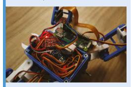
Attach battery and charging cables, Arduino and Arduino IO shield, and install the Arduino code before inserting Raspberry Pi Zero W, USB microphone, and Camera Module.
