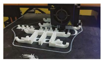
Arijit 3D-printed the parts for the spider robot's chassis
