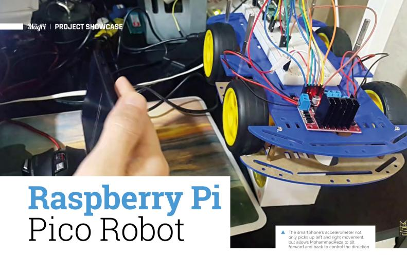
Rather than use a standard controller, this robot is steered using an Android phone's accelerometer. **David Crookes** takes a look
