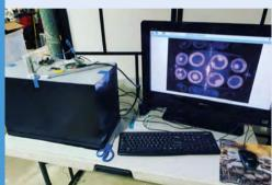
To start data collection, turn on the Raspberry Pi camera, start Python, and run main.py. If successful, the image loader will run on bootup next time.
