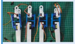
Download and 3D-print the spider body parts (magpi.cc/spyderprint). Then attach the servo motors for the legs, and assemble the rest of the body.
