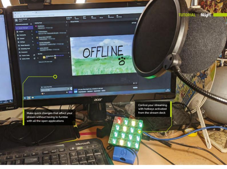
It's very quick to prototype and test your custom code as well - opening, editing, and then saving the **code.py** file will immediately reset Keybow 2040 so that you can test out your handiwork.
