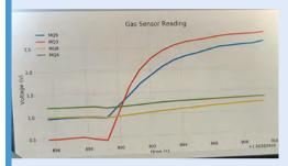
The sensors are calibrated when it turns on this is done by having the Python script run on start up, and holding the sensors away from anything you'd like to whiff. Once the sensors are calibrated to neutral, a sensor reading will be displayed.
