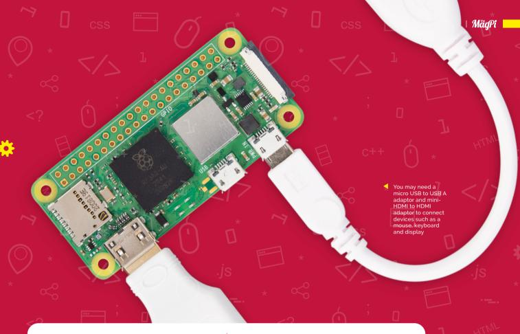
your Raspberry Pi Zero 2. Connect the other end of the HDMI cable to an HDMI monitor or television.
