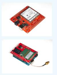
Two ways to get GPRS to a microcontroller: the Telit GM862 evaluation board breaks out all the pins of the module to 0.1" spacing; the SM5100B shield breaks out the serial pins of its module to the Arduino's serial pins.
