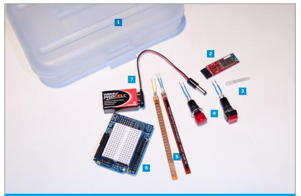
Figure 2-1. New parts for this chapter: 1. Project box 2. Bluetooth Mate 3. RGB LED 4. Pushbuttons 5. Flex sensors 6. Prototyping shield, 7. 9V battery snap connector and female power plug. Don't forget plenty of male header pins for the breakout boards.
