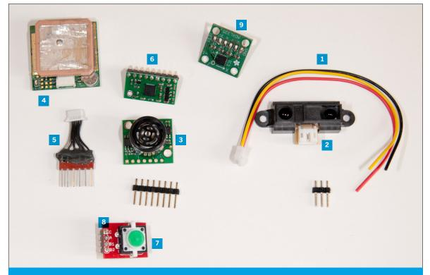
**Figure 8-1.** New parts for this chapter: **1.** Sharp GP20Y0A21 IR ranger **2.** JST pigtail for IR ranger **3.** Maxbotix LV-EZ1 ultrasonic ranger **4.** EM-406A GPS receiver **5.** Interface cable for EM-406A **6.** LMS303DLH digital compass **7.** LED tactile button **8.** Breakout board for button **9.** ADXL335 accelerometer. Don't forget plenty of male header pins for the breakout boards.
