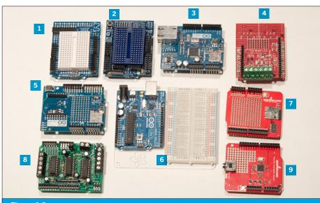
Figure 1-9. A sampling of shields for Arduino: 1. Arduino prototyping shield 2. Adafruit prototyping shield 3. Arduino Ethernet shield 4. TinkerKit DMX shield 5. Arduino wireless shield 6. Oomlout Arduino/breadboard mount, manufactured by Adafruit 7. Spark Fun microSD card shield 8. Adafruit motor driver shield 9. Spark Fun musical instrument shield.
