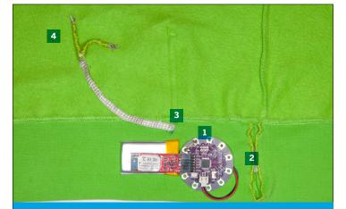
**Figure 10-21.** The layout of the hoodie components on the inner lining: 1. The LilyPad Arduino and the battery are actually inside the bottom band of the garment, inserted through 2. the large cut on the right. The conductive ribbon comes out of the bottom band through 3. the small cut, and goes to 4. the pocket contacts at the top (opposite side of the garment).
