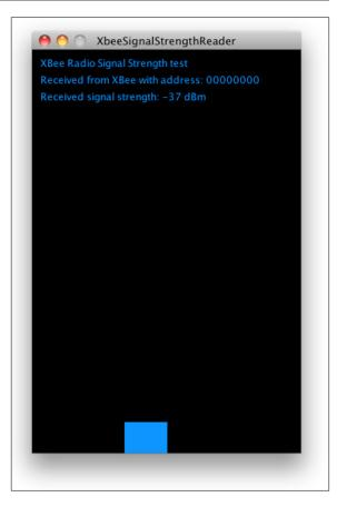
Figure 8-7 Output of the XBee RSSI test program.
