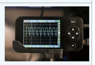
★ Figure 6-4. An oscilloscope can help you see the pattern of an IR signal.
