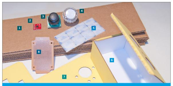
**Figure 5-1.** New parts for this chapter: **1.** Triple-wall cardboard **2.** 3-axis accelerometer **3.** 2-axis joystick **4.** Pushbutton **5.** Velcro **6.** Project enclosure, made from mat board **7.** 1/16" mat board template for project enclosure **8.** Perforated circuit board. Don't forget plenty of male header pins for the breakout boards.
