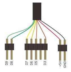
▲ Figure 9-21 The header pin connections for the cable to the perfboard.
