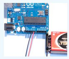
Figure 6-17 Arduino module powered by a 9V battery.
