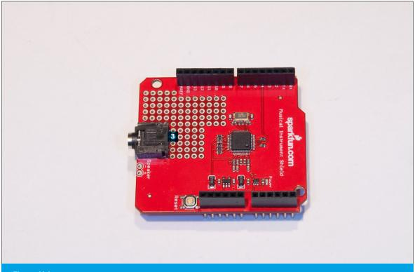
Figure 11-1. New parts for this chapter: Spark Fun Musical Instrument shield.
