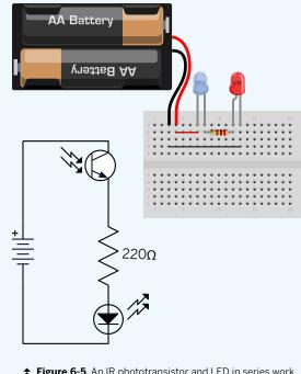
★ Figure 6-5. An IR phototransistor and LED in series work well to test IR reception.
