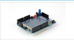
The ultimate open source prototyping shield for Arduino & compatible microcontrollers. Create your circuits the way you want, and easily changes without having to solder.
