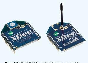
Figure 6-9. XBee 802.15.4 modules. XBee low-power module with chip antenna on the left, and XBee-PRO extended range module with wire antenna on the right. *Pictures courtesy of Digi International.*
