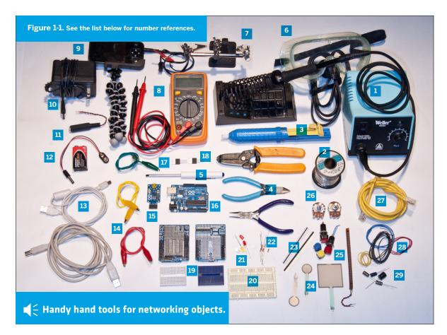
**1** Soldering iron Middle-of-the-line is best here. Cheap soldering irons die fast, but a mid-range iron like the Weller WLC-100 works great for small electronic work. Avoid the Cold Solder irons. They solder by creating a spark, and that spark can damage static-sensitive parts like microcontrollers. Jameco (http://jameco. com): 146595; Farnell (www.farnell.com): 1568159; RadioShack (http://radioshack. com): 640-2801 and 640-2078
