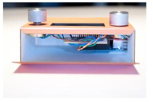
Figure 9-22 The inside of the box with the LCD perfboard in the foreground.
