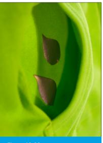
**Figure 10-22.** The conductive fabric contacts inside the hoodie pocket.
