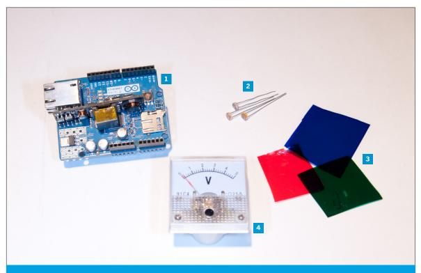
**Figure 4-1.** New parts for this chapter: **1.** Arduino Ethernet shield—this one has a Power over Ethernet module on board **2.** Photocells **3.** Red, green, and blue lighting filter gels **4.** Voltmeter. You can use an off-the-shelf one, but it's better if you can find one that's antique. Don't forget plenty of male header pins for the breakout boards.
