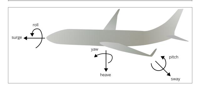
**Figure 8-14** Rotations and translations of a body in three dimensions.
