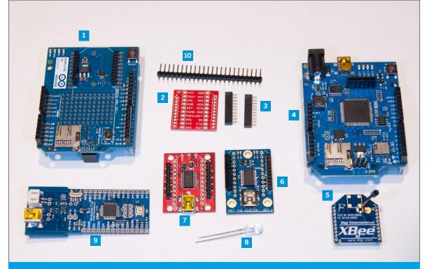
**Figure 6-1.** New parts for this chapter: **1.** Arduino wireless shield **2.** Spark Fun XBee breakout board **3.** 2mm female header pins **4.** Arduino WiFi shield **5.** Digi XBee 802.15.4 OEM module **6.** Adafruit XBee-to-USB adapter **7.** Spark Fun XBee Explorer **8.** Infrared LED **9.** Arduno Fio. Don't forget plenty of male header pins for the breakout boards.
