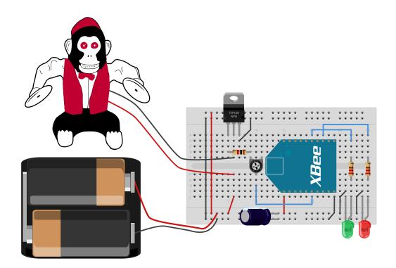
**Figure 7-6** XBee radio connected to a cymbal monkey.
