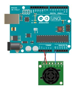
This sketch is similar to the infrared ranging sketch in Project 15. It reads the sensor and converts the results to a voltage, then converts that to a distance measured in centimeters. The conversion formula again gives only an approximation.
