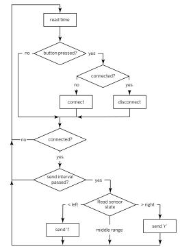
Figure 5-2 Logic flowchart for the pong clients
