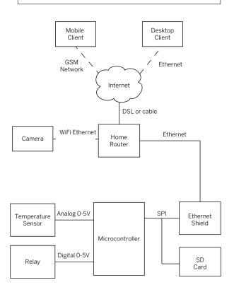
communicates with the microcontroller via SPI, as does the SD card on the shield or board. The temperature sensor is an analog input, and the 120V relay to control the air conditioner is a digital output. The IP camera in this project is a consumer item that has a built-in server, so all you have to do is configure it to speak to your router. The clients are just web browsers on your smartphone, tablet, or personal computer.
