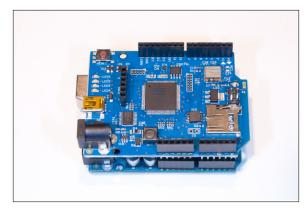
Figure 6-22 Arduino WiFi shield.
