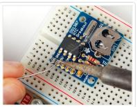
If you'd like to use the header to plug the breakout board into something, place the header in a breadboard, long side down and place the board so that the short pins stick thru the pads.
