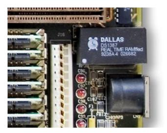
The image above shows a computer motherboard with a Real Time Clock called the DS1387 (http://adafru.it/aX0). There's a lithium battery in there which is why it's so big.
