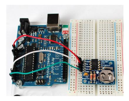
If you set analog pin 3 (digital 17) to an OUTPUT and HIGH and analog pin 2 (digital 16) to an OUTPUT and LOW you can power the RTC directly from the pins!
