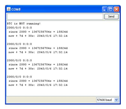
Whenever the RTC chip loses all power (including the backup battery) it will report the time as 0:0:0 and it won't count seconds (its stopped). Whenever you set the time, this will kick start the clock ticking. So basically the upshot here is that you should never ever remove the battery once you've set the time. You shouldn't have to and the battery holder is very snug so unless the board is crushed, the battery wont 'fall out'
