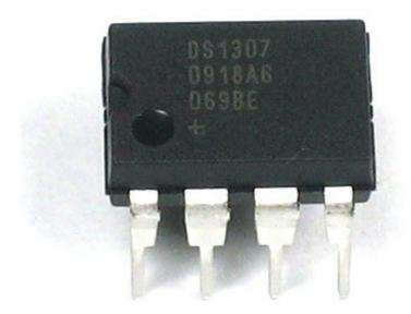
As long as it has a coin cell to run it, the DS1307 will merrily tick along for a long time, even when the Arduino loses power, or is reprogrammed.
