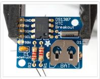
Place the two 2.2K resistors, and the ceramic capacitor. They are symmetric so no need to worry about direction.
