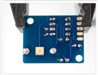
Clip the leads of the resistors, crystal and capacitor short.
