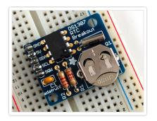
Insert the battery so that the flat + side is UP. The battery will last for many years, 5 or more, so no need to ever remove or replace it.
