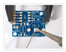
Begin by soldering a small bump onto the negative pad of the battery: this will make better contact!
